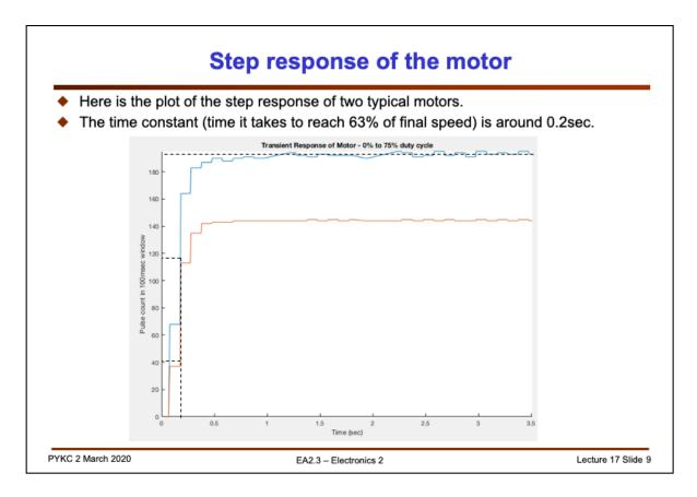
I also test the response of the motors to a step input (going from PWM=0% to 75%).
